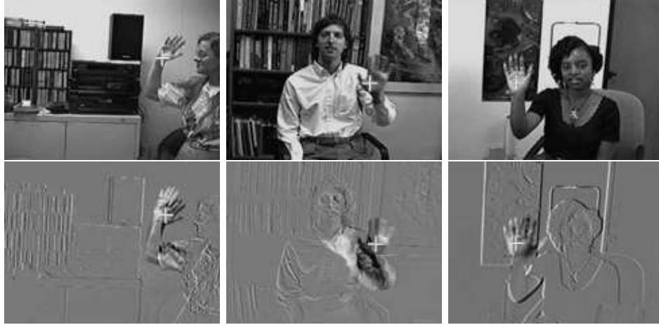
Figure 5: Sample video frames used by the hand tracking subsystem. The upper frames are used by the intensity pathway. The lower frames are corresponding difference images used by the difference pathway. The white cross indicates the position of the hand predicted by the network.
